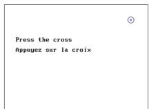
Calibration is important for user comfort. It is strongly recommended to perform it by placing the device on a table and using the stylus.
